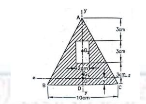
16. Support A has ball and socket connection. Roller support at B prevents motion in the -z direction. Corner *C* is tied to *D* by a rope. The triangle is weightless. Determine the unknown force components acting at *A*, *B*, and *C*. (14 marks)
